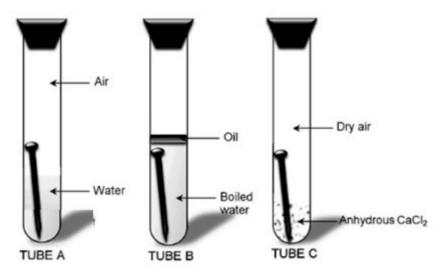
In which test tube nail is rusted?
